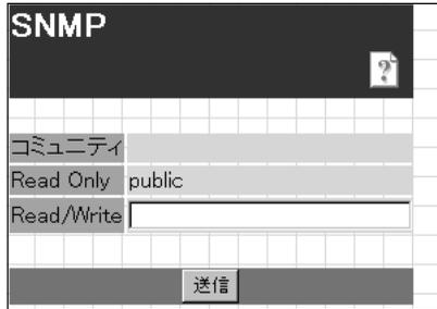
The image shows a web-based configuration form for SNMP Community. The title is "SNMP". There are three input fields: "コミュニティ" (Community) with a greyed-out field, "Read Only" with the value "public", and "Read/Write" with an empty text box. A "送信" (Send) button is at the bottom.
