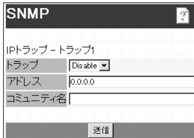
The image shows a web-based configuration form for SNMP IP Trap. The title is "SNMP". The sub-title is "IPトラップ - トラップ1". There are three input fields: "トラップ" (Trap) with a dropdown menu set to "Disable", "アドレス" (Address) with the value "0.0.0.0", and "コミュニティ名" (Community Name) with an empty text box. A "送信" (Send) button is at the bottom.
