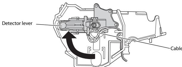
5. Tighten the detector adjustment screw.
