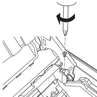
9. Tighten the screw ( $3 \times 10$ ) to fix the roll paper holder for hanging bracket and the roll paper holder.
