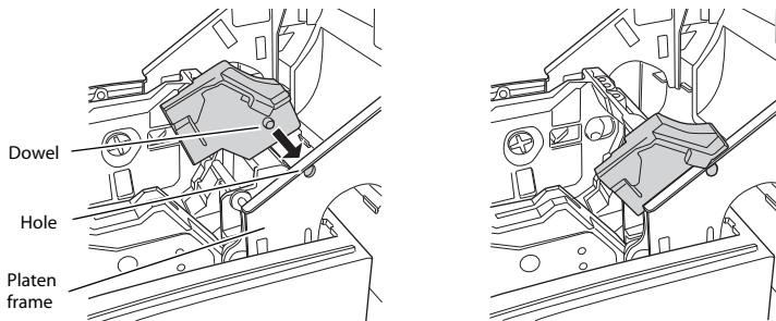
12. While you make sure the pin of the brake arm is in the groove on the inner side of the cam, rotate the cam along with the surface of the platen frame in the direction indicated by the arrow until it clicks into position.
