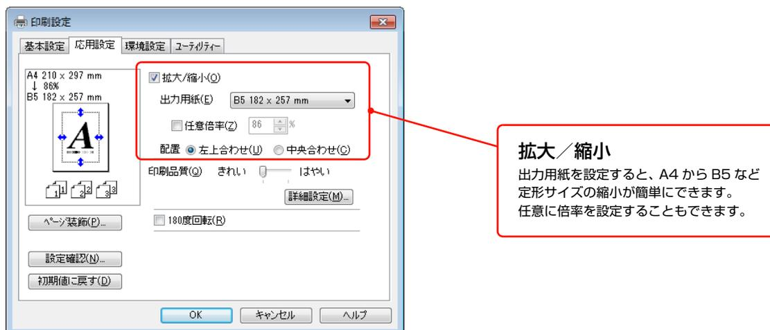
The screenshot shows the '印刷設定' (Print Settings) dialog box with the '応用設定' (Advanced Settings) tab selected. A callout points to the '拡大/縮小' (Scale) section:
