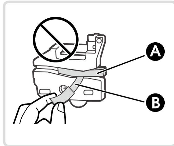
**EN** Replace the cutter without removing the protective material (A) and protective tape (B) that are stuck to the cutter blade.
