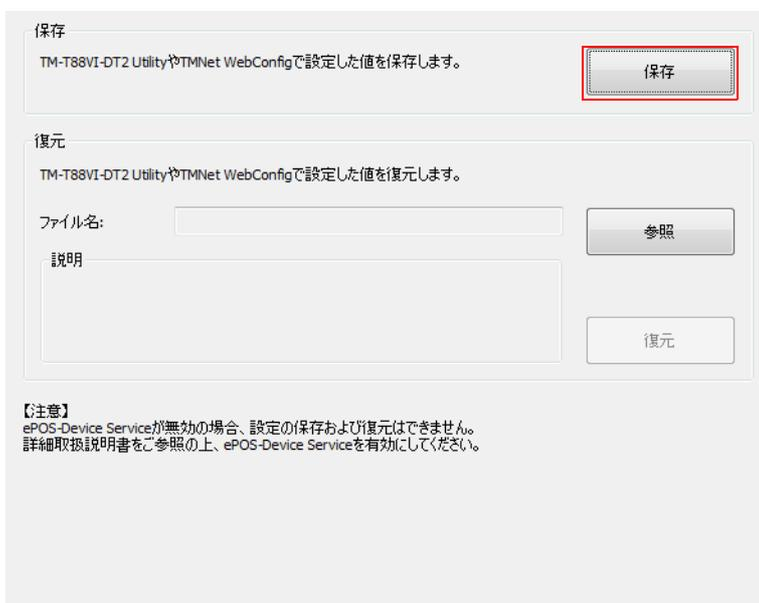
The screenshot shows a dialog box with two main sections: '保存' (Save) and '復元' (Restore). The '保存' section contains the text 'TM-T88VI-DT2 UtilityやTMNet WebConfigで設定した値を保存します。' and a '保存' button. The '復元' section contains the text 'TM-T88VI-DT2 UtilityやTMNet WebConfigで設定した値を復元します。', a 'ファイル名:' label with an input field, a '参照' button, a '説明' label with a text area, and a '復元' button. At the bottom, there is a '【注意】' (Note) section with a warning message about ePOS-Device Service.
